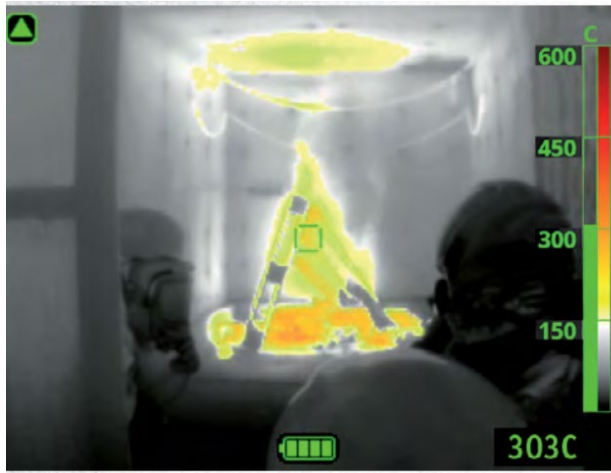
Figure 3-18 X-Factor Lite Image Enhancement Image Credit: Bullard
