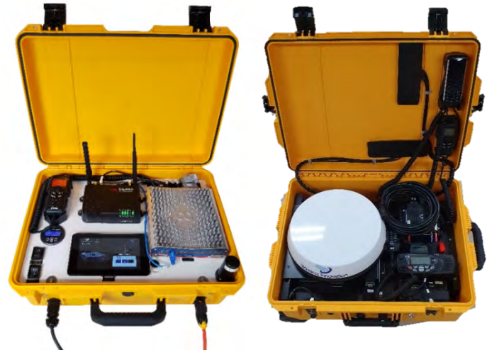
Figure 3-20 Portable Radio Repeater Deployment Kit without SATCOM interface (left) and with SATCOM interface (right)
