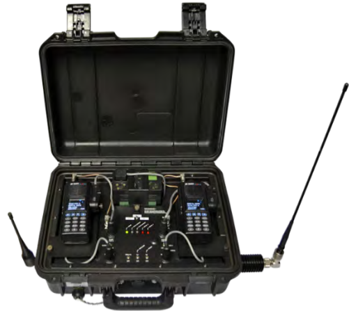
Figure 3-3 Rapid Deployment Portable Repeater Courtesy of BK Technologies
